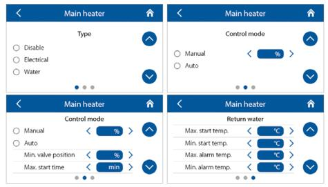
Select the heater type and set up its parameters.
