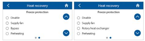
**Freeze protection** — type of heat exchanger freeze protection.
